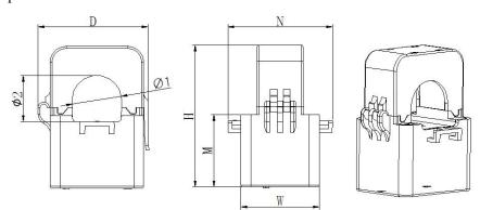
The transformers' secondary outlet wire is single RV lead, whose standard length is  $2m(\pm 10cm \text{ error allowed})$ .
